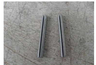
Replacement Roll Pins. 50mm x 6mm
